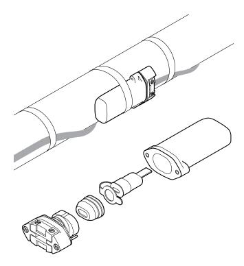
The JQH-LEC is a cold applied low profile end seal. This universal end seal is designed to fit with all Santo industrial self-regulating heating cables; UFA, UFB, UFC and UFO meaning simplified product selection and reduced inventory to stock. It can be used in applications with temperatures ranging from -50°C to 215°C. It is approved for use in hazardous areas.
