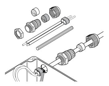
This connection kit is designed for terminating all Santo UFA, UFB, UFC, UFO and ACC industrial parallel heating cables to a junction box, whilst maintaining electrical insulation of the heating cable conductors and core. It is approved for use in hazardous areas.
