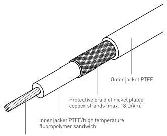
High temperature resistance heating conductor
